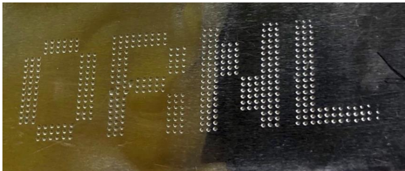
Inkjet printing of Targets: Successful Printing of Bitmap Patterns: 50 nL drops of water on aluminum
