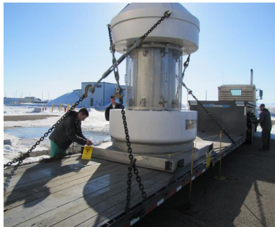
Co-60 loaded in BRR Cask for shipment to a commercial vendor; first use of the BRR Cask
