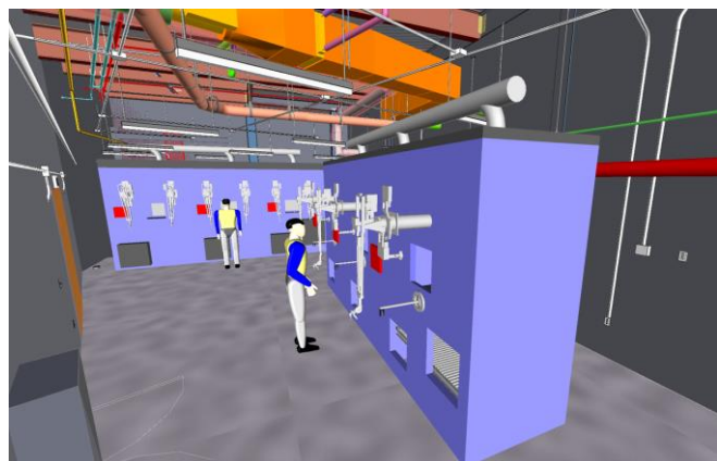
Conceptual view of new hot cells for purifying and harvesting the radioisotopes from the FRIB beam dump system.
