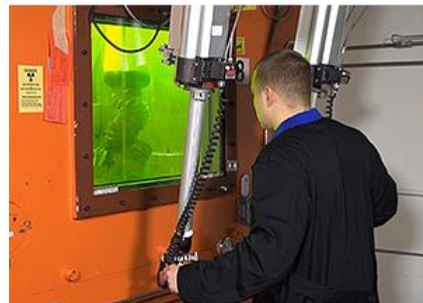
Hot cell work on Sr-90 conversion and purification
