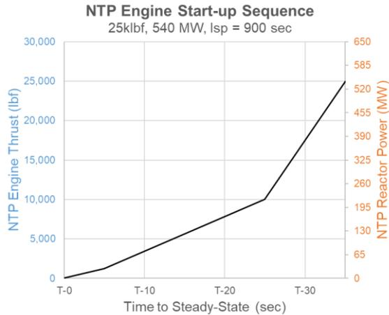
**Figure 3 – NTP Engine Start-Up Sequence**
