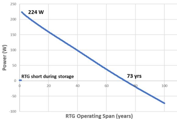
Figure 4. GPHS-RTG power prediction for ISP through 100 years with 16 GPHS
