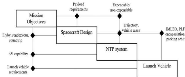
**Fig. 2.** Mission design problem for NTP powered missions.
