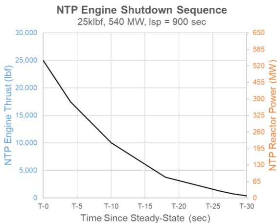
**Figure 4 – NTP Engine Shutdown Sequence**
