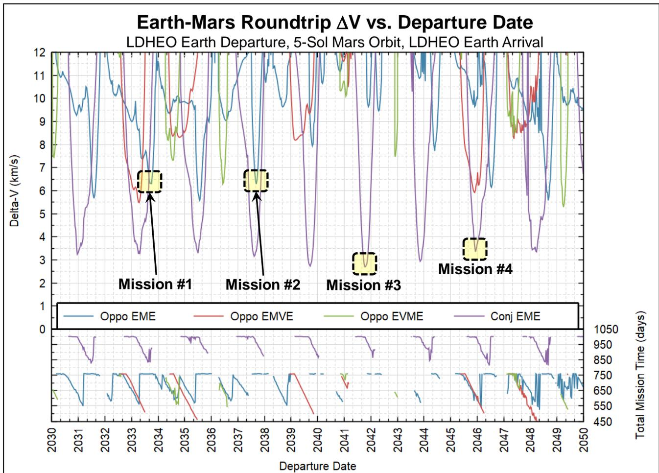
**Fig. 1.** Roundtrip Mission  $\Delta V$  for Mars Conjunction and Opposition Missions from 2030-2050
