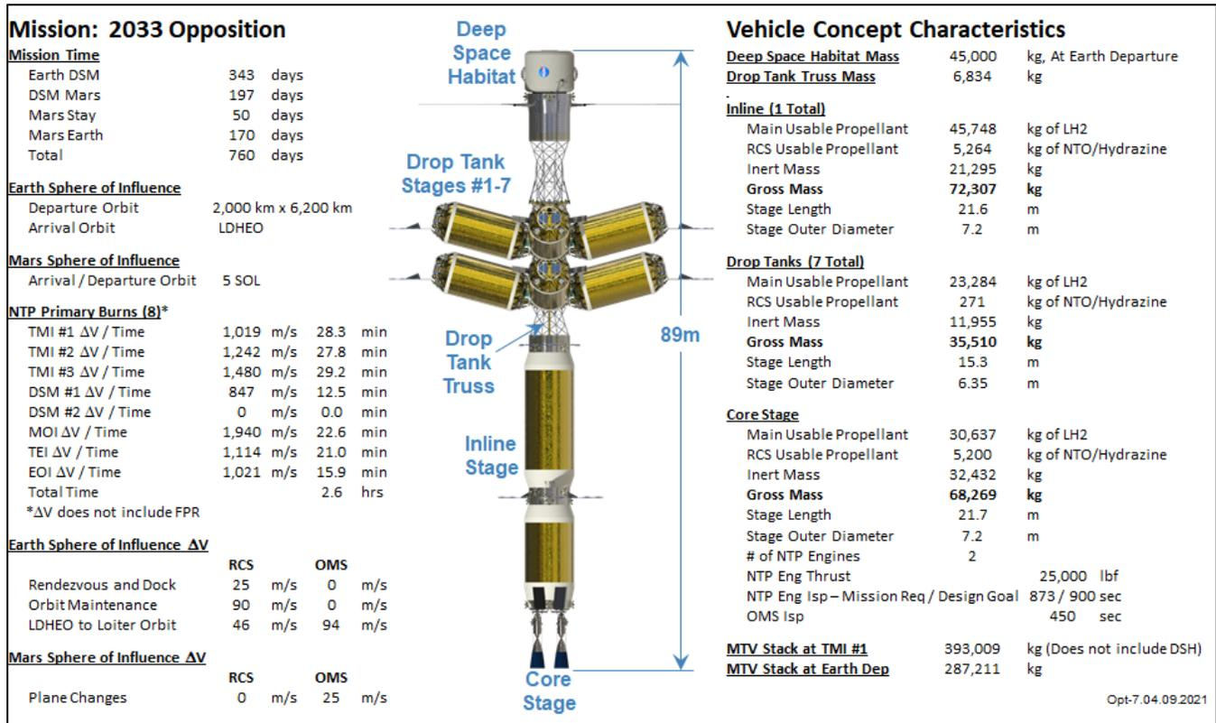
Fig. 4. Mars Transport Vehicle Details for Cis lunar and Mars Flight Demonstration Missions
