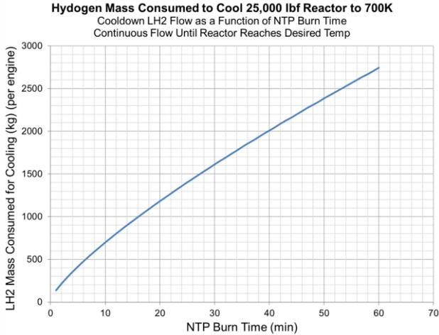
**Figure 5 - NTP Cooldown Flow per Engine Burn Time**
