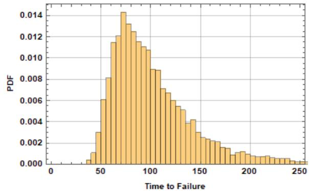
**Figure 3. Bayesian assessment shows RPS time to failure distribution**
