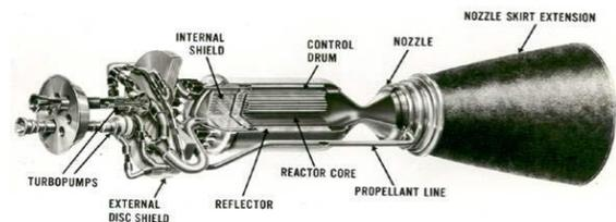
**Fig. 1.** Schematic of an NTP engine [7].
