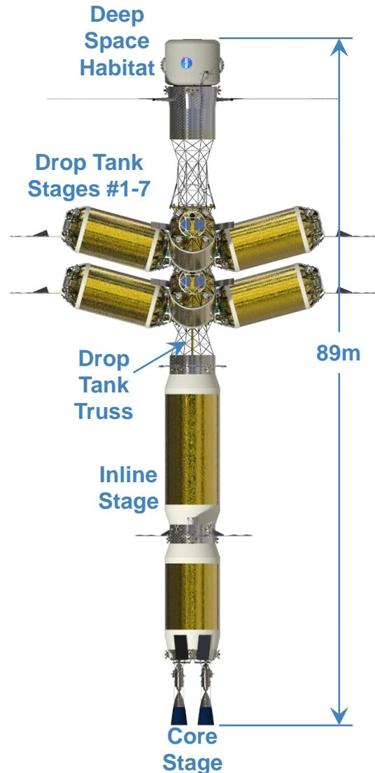
**Fig. 2.** Mars Transport Vehicle for Cislunar and Mars Flight Demonstration Missions
