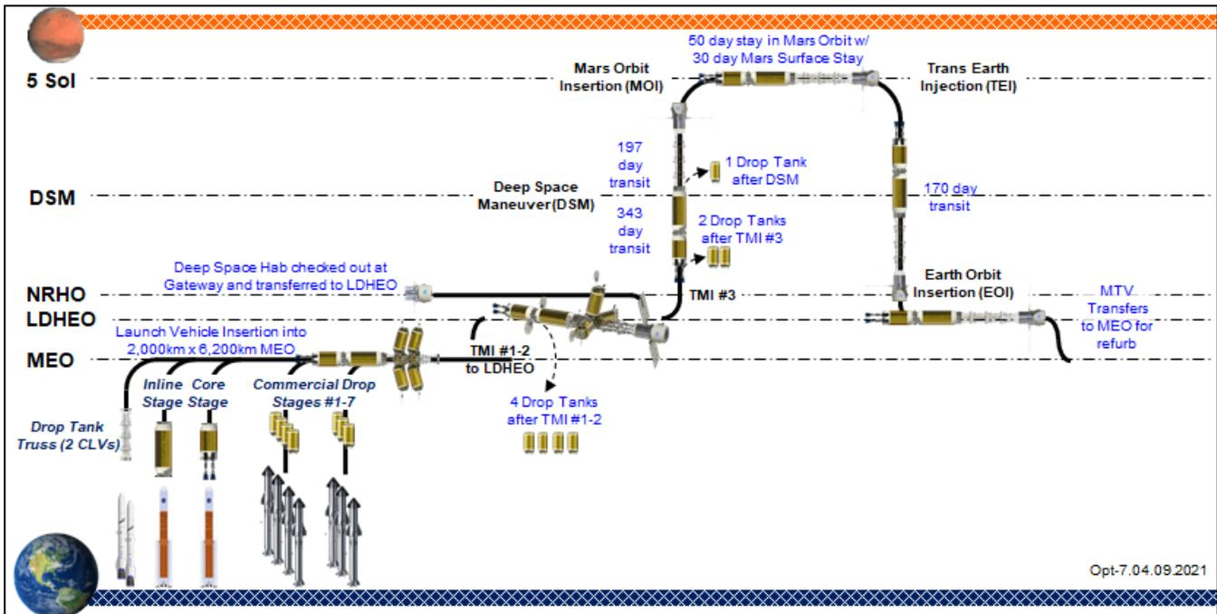
Fig. 3. Concept of Operations for Cislunar and Mars Flight Demonstration Missions
