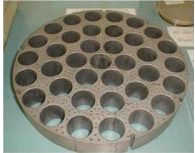
Fig. 7. ZrH block used for the RD-0410 moderator 5
