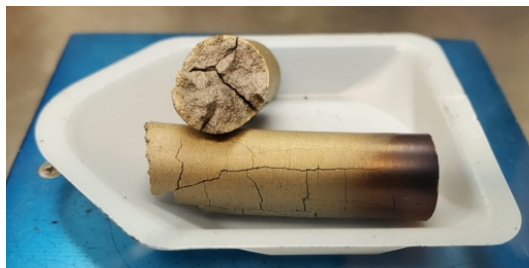
Fig. 2. ZrH as Manufactured Through Direct Hydride Method
