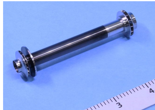
Fig 2. Rotor assembly with compressor impeller and thrust bearing disk (left) and turbine impeller (right).
