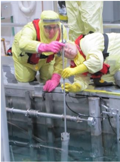
Fig. 8. ATR Canal Operators load a basket containing a PFS target into the South Irradiation Housing Assembly
