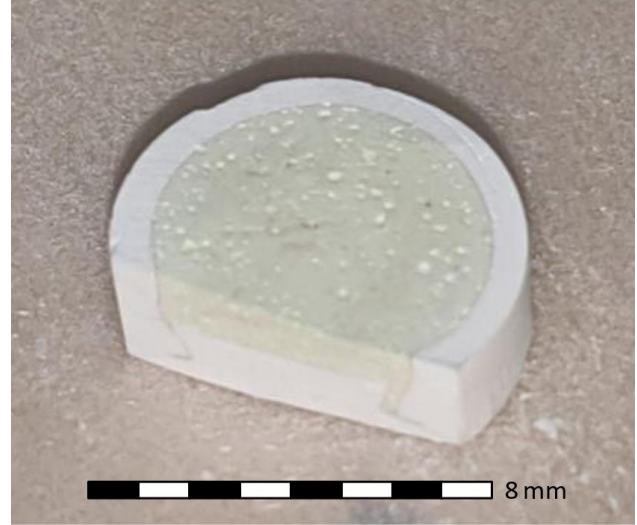
Fig. 5. Sectioned thulium CAB unit prototype after sintering, showing internal layered structure.
