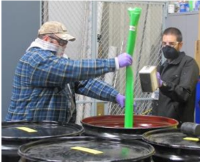
Fig. 7. ATR Personnel remove a PFS-3 target from the shipping drum while monitoring radiation levels.
