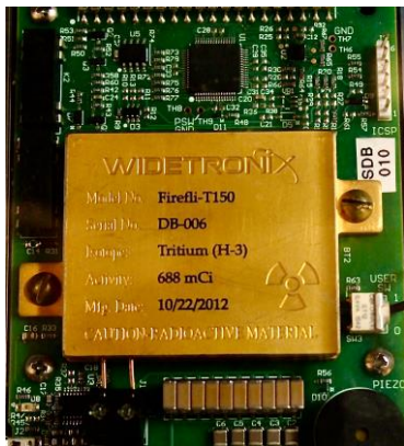
Fig. 6. Widtronix Firefli betavoltaic. It is made up of tritium isotope sources and SiC converters.
