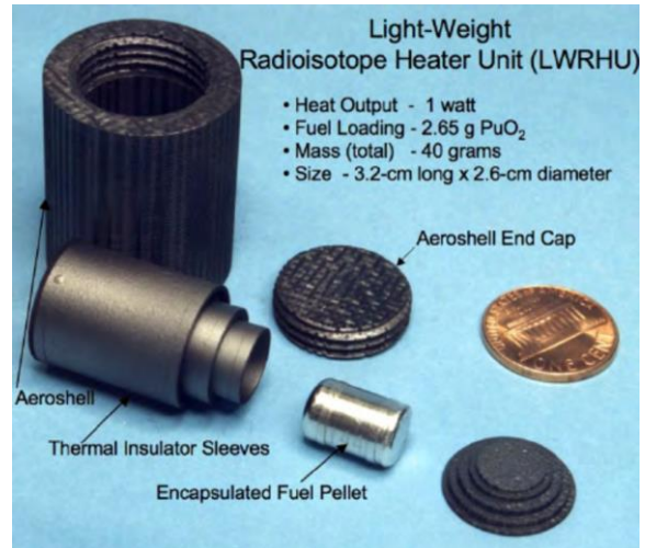
Fig 1. Photograph of watt-scale RHU components with penny for scale. 1
