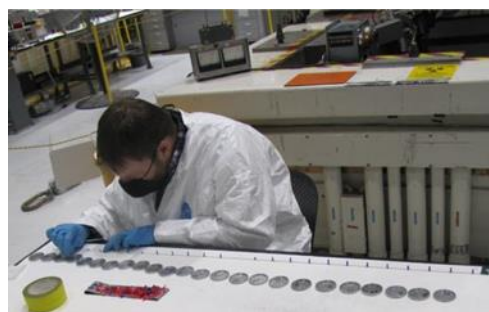
Fig. 6. ATRC facility personnel remove and arrange irradiated flux wires for analysis
