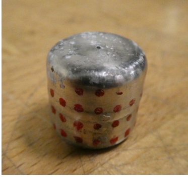
Fig. 2. Pt-30Rh RHU clad, end-on impact
