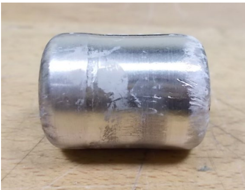
Fig. 3. Pt-20Rh RHU clad, impacted twice end-on
